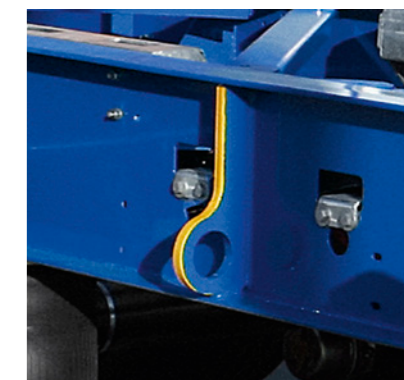
The container trailer chassis can be equipped with ferry lashings* for use with ferry transport.
