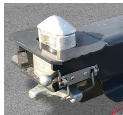
Standard TWIST LOCK locking mechanism: lowerable and with anti-twist device.
