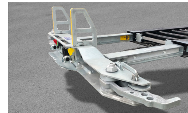
The front extension for 45' containers is spring-mounted on roller bearings, providing simple, safe and rapid handling.
