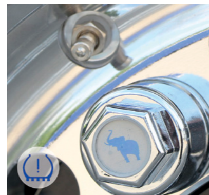
Integrated tyre pressure control system: the correct tyre pressure reduces tyre wear and lowers fuel costs due to better roll resistance
