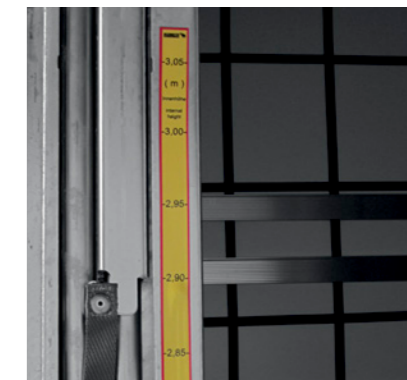
VARIOS body: height adjustment in 50 mm increments at the bulkhead from 2,700 to 3,050mm and at the rear portal from 2,850 to 3,050 mm. Ideal for switching to different semi-trailer heights./***
