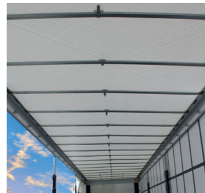
Schmitz Cargobull safety roof with built-in diagonal reinforcement increases structural rigidity.
