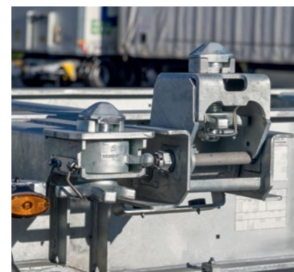
With 2 x 20' loads, the height-adjustable KLAPP LOCK takes over the locking of the front container.
