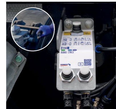
Control unit for pneumatic locking for the rear extension, optionally with manual locking*.
