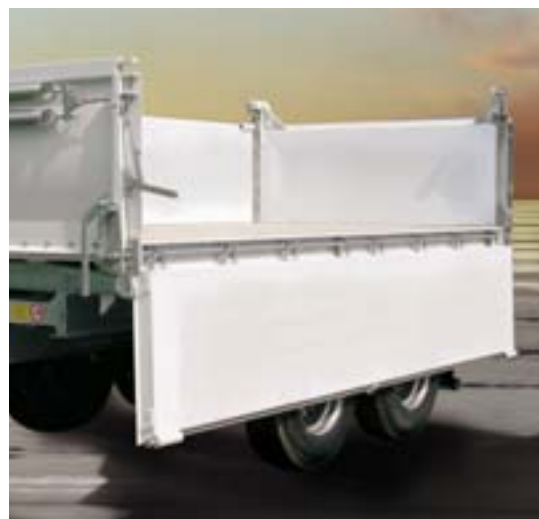
Without middle stanchions: The folded down bulkhead provides optimal access to the tipping bridge.
