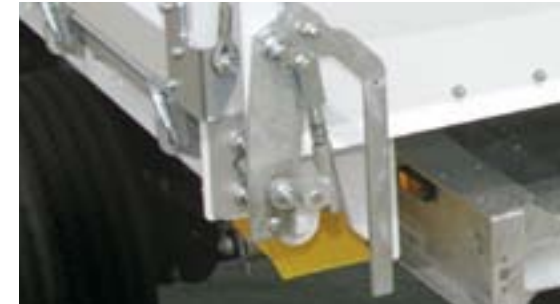
The aluminium side walls can be opened and closed conveniently with the side wall raising aid on both sides.
