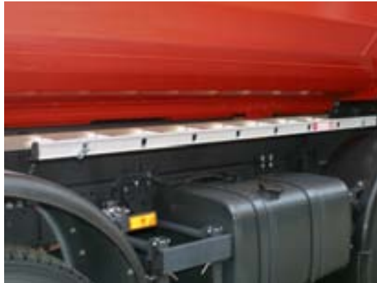
The sensible option: The light-weight aluminium ladder is mounted above the mudguard using two clips.
