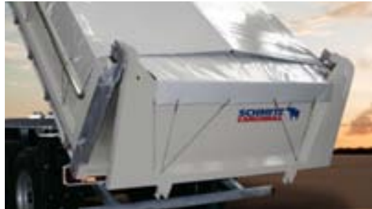
The divided rollup tarpaulin with the attached rear tarpaulin section for legally required load securing. The roof design is stabilised by a longitudinal member.
