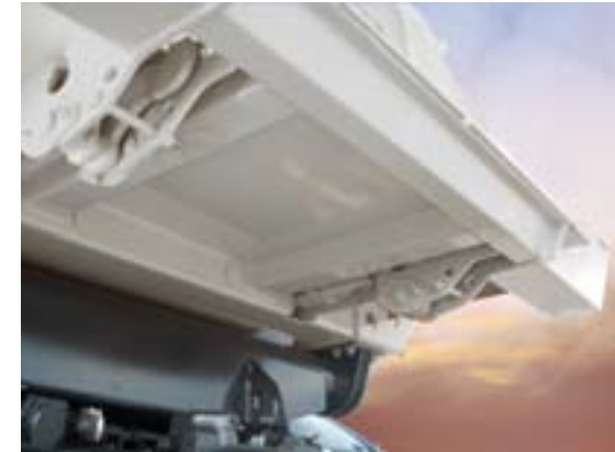
The durable draw hooks on the tailgate are guided by a robust rods.
