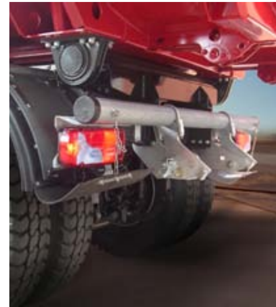
Underride guard folded up for unloading close to the road paver.
