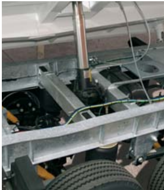
The hot galvanized, welded steel frame ensures a long service life.
