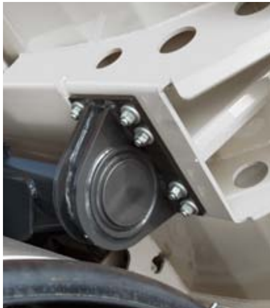
The tipping bearings on the body of a long service life and require little maintenance.
