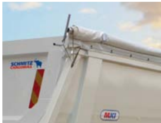
The rollup tarpaulin covers the body flush with the lip and secures the load against the influence of the wind.
