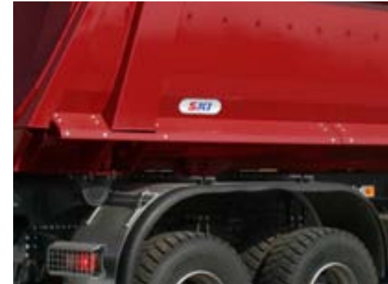
Side fender plates on the rounded steel body protect the running gear when loading.
