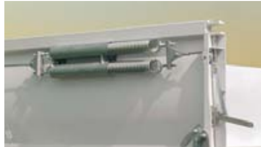
The central lock for the pendulum-mounted side walls on the front bulkhead possesses an over-centre helper spring for rapid, safe locking.
