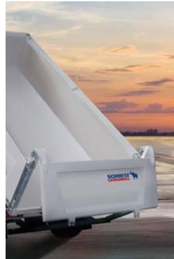
The rear wall with the top-mounted pendulum bearing creates a large opening cross-section.
