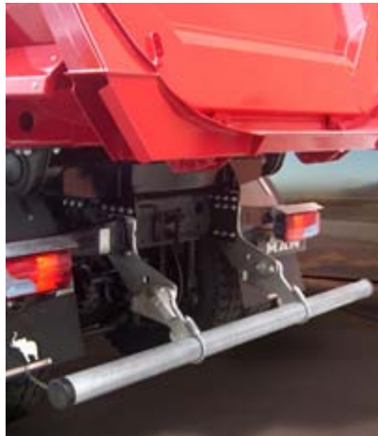
The robust underride guard is weight-optimised and folds up easily.
