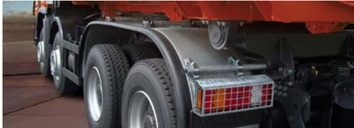
The bracket for the integrated mudguard is mounted directly onto the subframe. The optional rear light protective gratings are made of corrosion-resistant steel.
