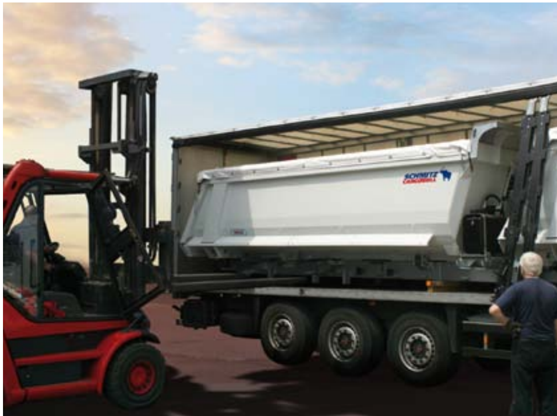
On the way to the vehicle assembler: Tipper body as an assembly-ready kit.
