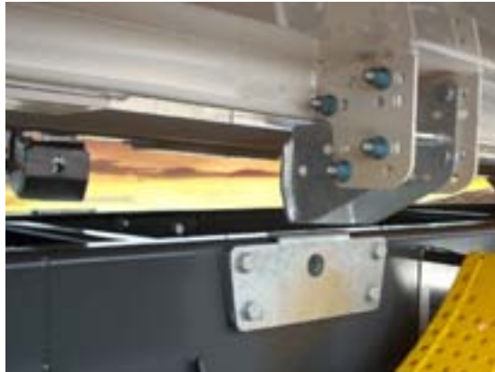
The body position guide serves to guide the body into the right position while lowering the body when the vehicle is inclined sideways.
