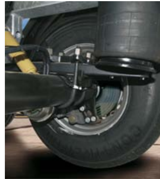
The axle unit with air suspension and EBS is available with either disc brakes or drum brakes.
