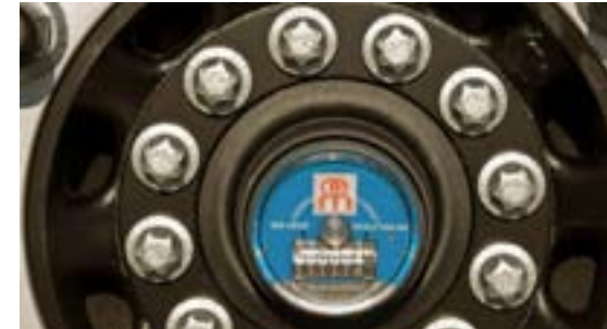
The odometer provides you with a reliable overview of the mileage.
