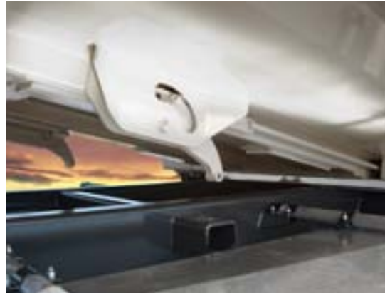
The mechanical locking hooks on the pendulum tailgate lock automatically.
