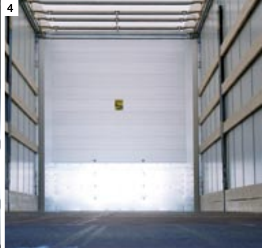
4. Bulkhead from hollow section (anodized) aluminium with ramming protection made from 750 mm high galvanised steel plate.
