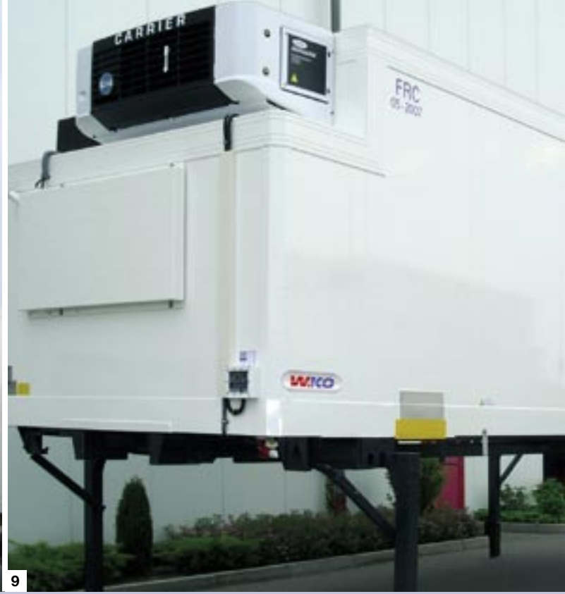
9. W.KO 7.45 FP 80/60 NB with FERROPLAST construction and chiller for frozen goods transport.
