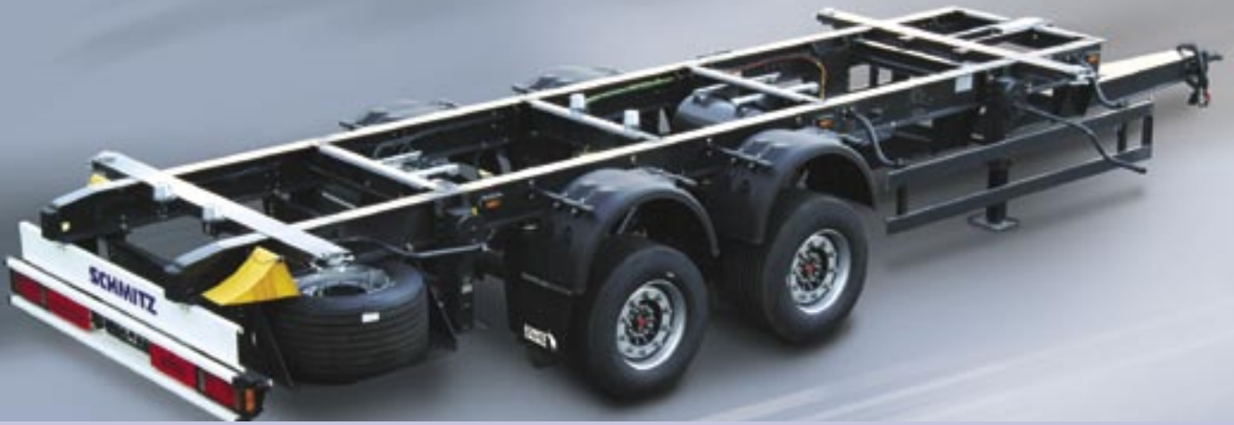
5. Central axis chassis for swap container A.WF 18 maxi with 435/50 R19.5 tyres.
