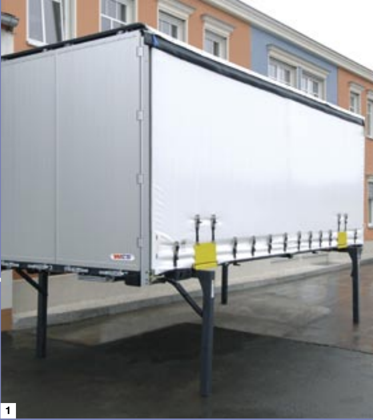
1. W.CS 7.45 swap curtainsider rail loading model.
