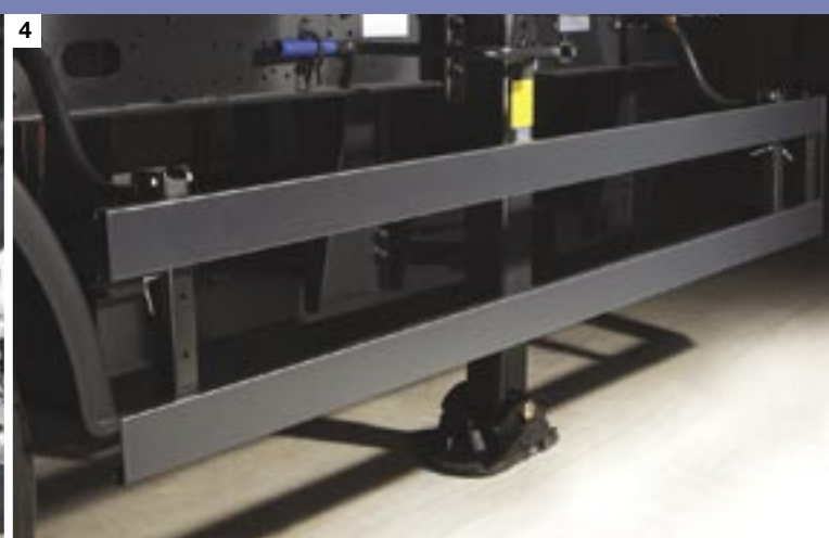
4. Front winding mechanism support attached to the frame on both sides with single sided operation or the right side, compensating foot and two gears.
