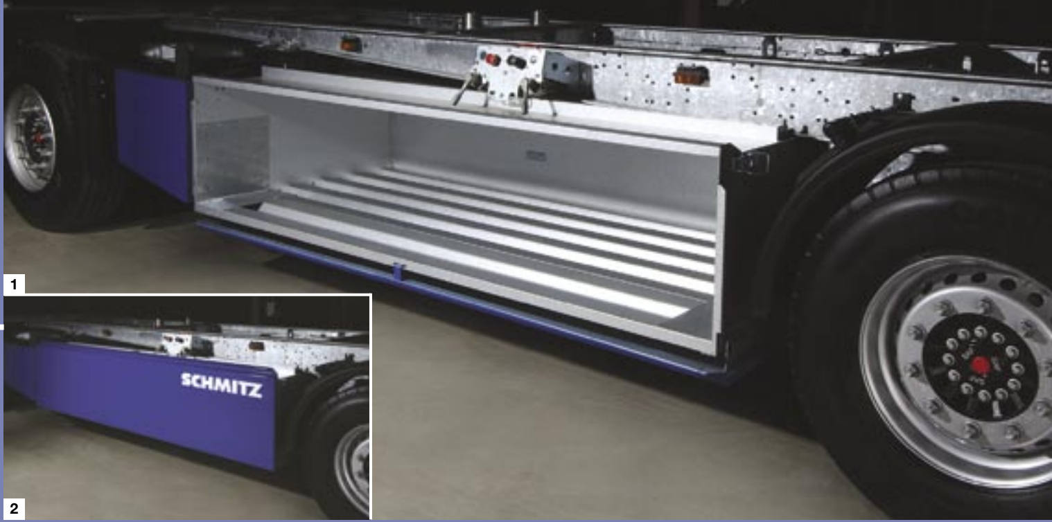
1. - 2. Closed model, galvanized pallet box.
