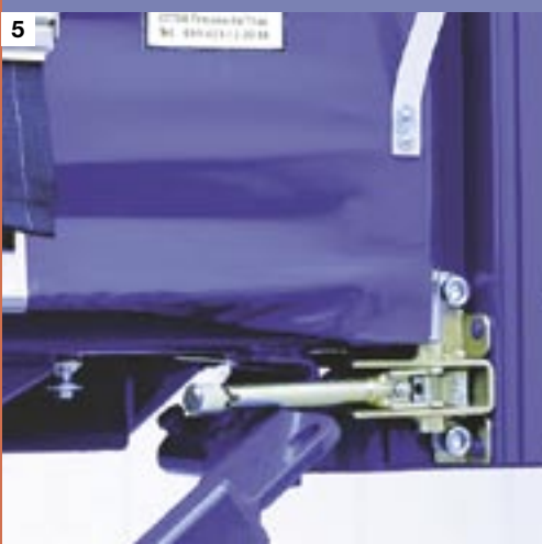
5. Tarpaulin tensioning using ratchet tensioning gear.
