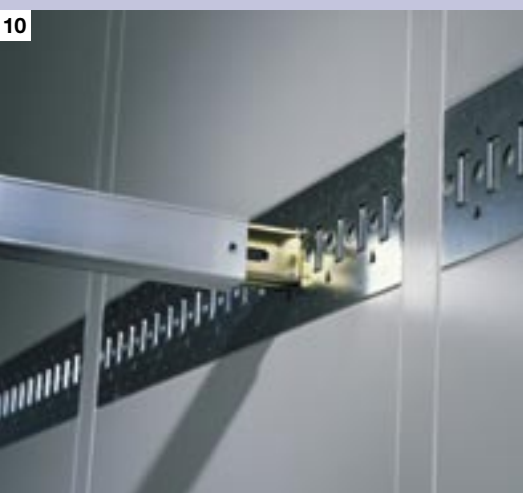
10. Loading securing rails integrated in side walls.
