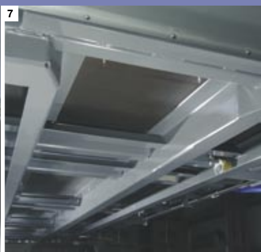
7. Stable floor construction with centring tunnel.
