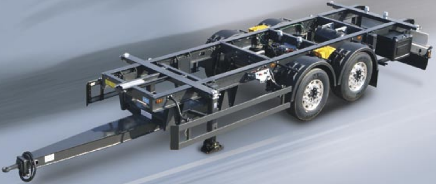
4. Central axis chassis for swap container A.WF 18 with 385/65 R22.5 tyres.
