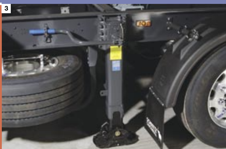
3. Rear winding mechanism support attached to the frame on both sides with single sided operation or the right side, compensating foot and two gears.
