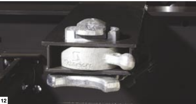
10. Galvanized guide rollers attached in mounting positions behind the rear container beam.
