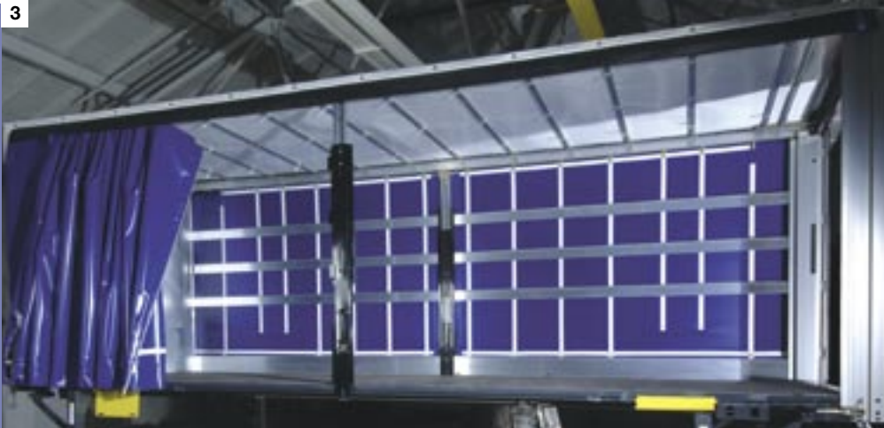
3. Side sliding tarpaulin with moveable posts and insertable aluminium slats.
