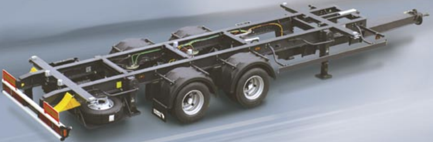
6. Central axis chassis for swap container A.WF 18 V with 235/75 R17.5 tyres.
