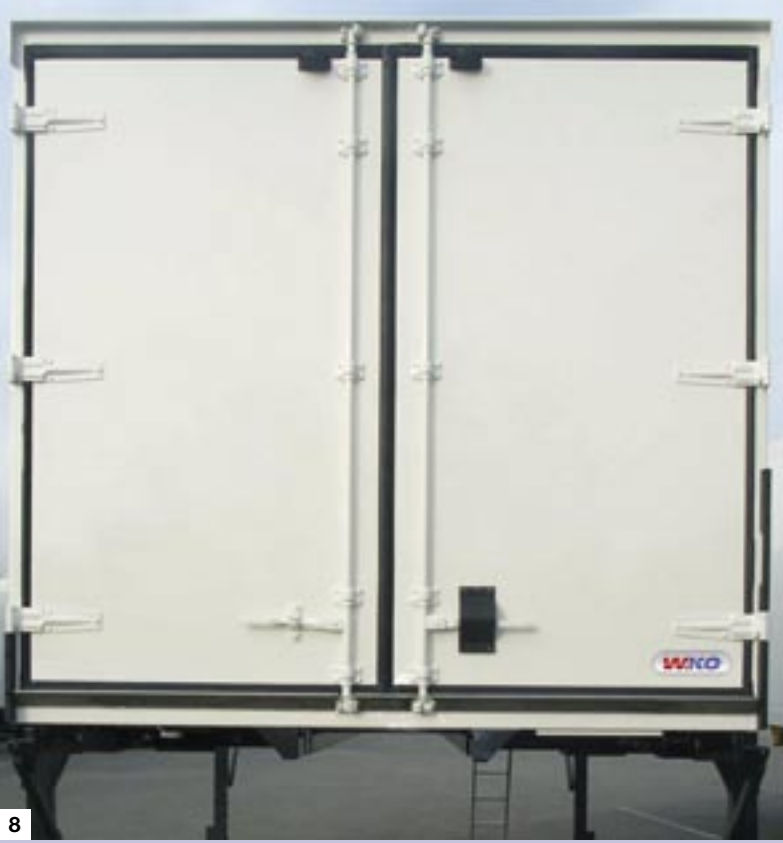
8. W.KO 7.45 FP 25 with FERROPLAST construction for dry freight, rear panel door.
