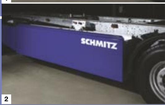
1. - 2. Closed model, galvanized pallet box.
