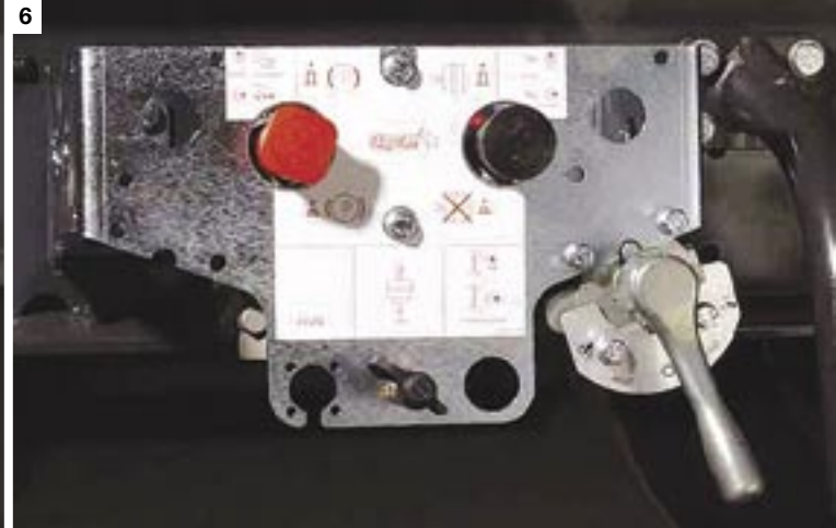
6. Control unit for park brake and air suspension with 1 lifting & lowering valve mounted on the side of the Z.WF longitudinal member.
