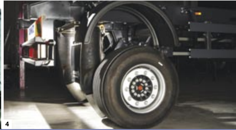
2. Undercarriage with drum brakes.
