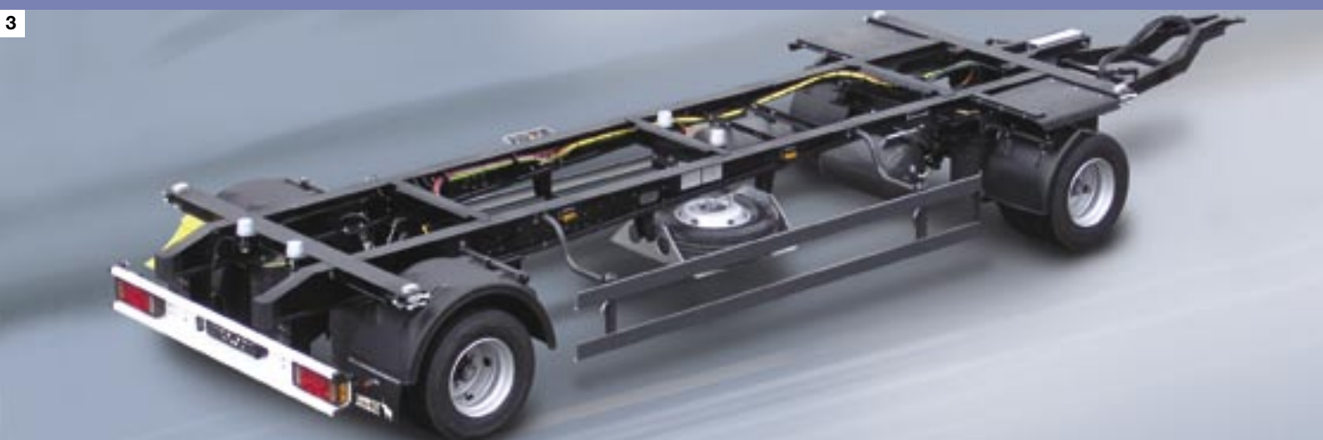
3. Trailer chassis for swap container A.WF 18 V with 235/75 R17.5 tyres.
