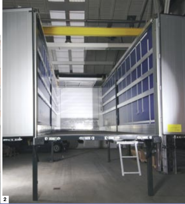
2. Schmitz Cargobull sliding tarpaulin. Pull-out dismounting ladder attached on rear right.
