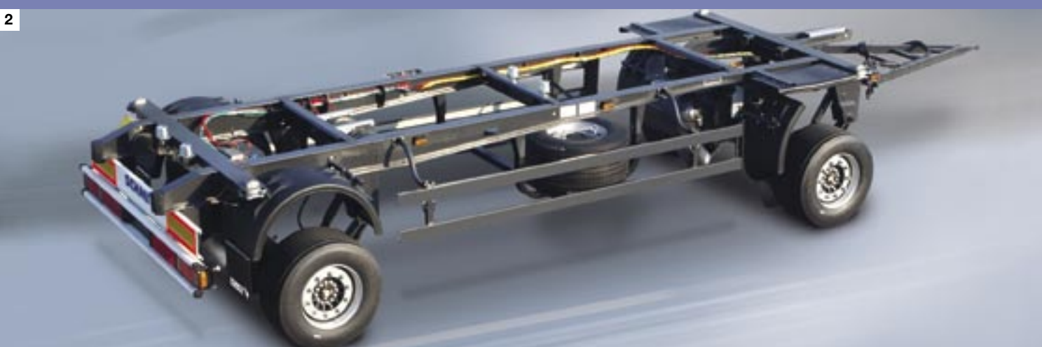
2. Trailer chassis for swap container A.WF 18 maxi with 435/50 R19.5 tyres in raised position.
