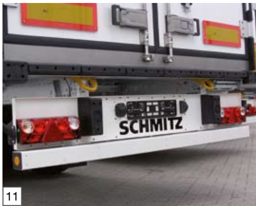
Barre anti-encastrement vissée
