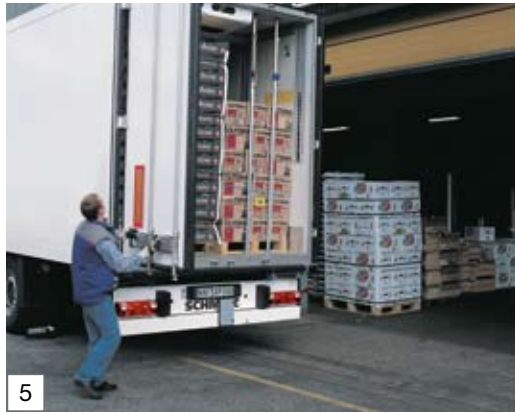
Door leaves can be pivoted through 270°
