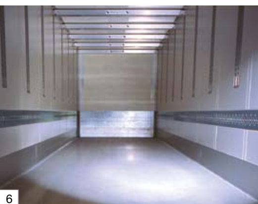
Combination of double deck loading and load securing system.
