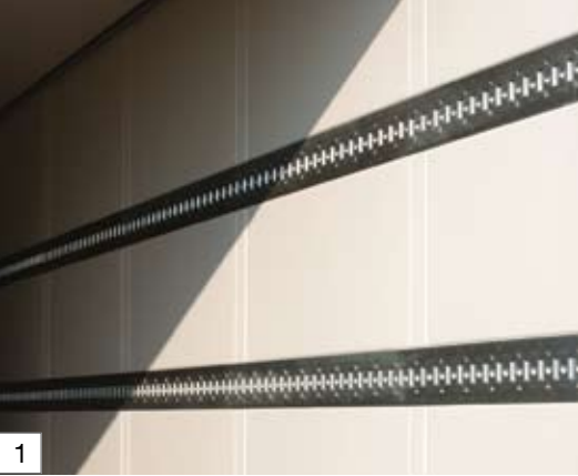
Additional load securing rails inlet in the side walls
