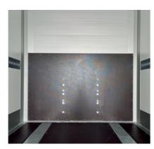
Aluminium front wall with laminated wood panel\*: Protection for cargo and trailer.
