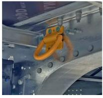
**Combined transport:** ferry lashings on the l-beams for short-distance sea transport.
