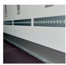
Flush load securing rails\* for horizontal beams, tensioning straps and securing tarpaulin.
