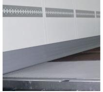
Durable and robust screen-printed floor up to 8,000 kg\* forklift axle load according to DIN 283. Sealed floor plates prevent moisture from reaching the cargo from below. Recessed wear plate\* protects the floor at the rear.
