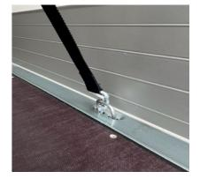
**External steel frame** with 16 pairs of recessed lashing eyes for load securing.
