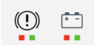
The two status LEDs indicate whether the immobilizer can be activated. This is the case when both LEDs light up green.
