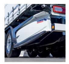
The lightweight and aerodynamically shaped stowage box\*\* ensures optimized air flow and contributes to further fuel savings. The large storage space offers room for pallets, spare wheels, etc.
