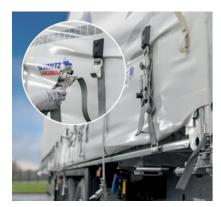
Quick flexible adjustment of the side tarpaulin on EcoFLEX and EcoVARIOS allows for an easy interchange of aerodynamic rear to full load volume
