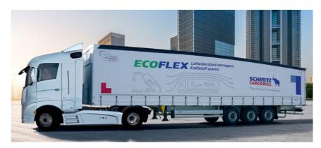
Efficient fuel reduction: The aerodynamic rear reduces the drag via a smaller surface and less vortex formation, allowing for greater airflow behind the vehicle.
