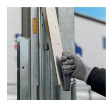
Simple handling via proven trailer technology: The rear height adjustment can be operated within minutes, in a similar way to our VARIOS height adjustable bodies, but without additional
