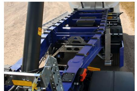
The **torsion-resistant steel chassis** with improved corrosion protection in a painted or galvanised finish ensures the best possible value retention.
