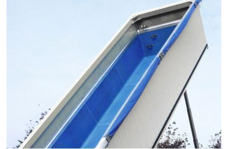
The **plastic lining\*** protects against wear, offers good sliding properties and reduces the risk of freezing.
