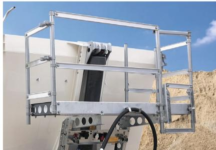
The **working platform** is used to operate the roller curtain and is equipped with a non-slip floor, body entry aid and parking position for the hydraulic hose.
