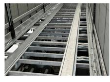
X-TOUGH chassis with high bending and torsional strength for 44 tonnes or more The S.CS X-TOUGH chassis impresses with its high bending and torsional strength. With its higher distributed load, optimised weight and a cross member spacing of max. 400mm, the MODULOS chassis offers greater strength reserves.
