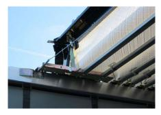
Schmitz Cargobull Safety Roof: Integrated diagonal bracing increases body strength.
