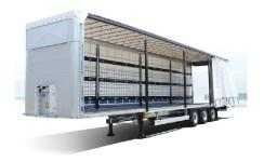
Standard body: The curtainsider's standard curtain is very smooth-running and can be opened and closed quickly and easily with just one hand.
