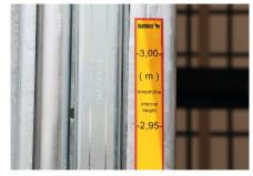
The height-adjustable VARIOS body ensures simpler and more flexible dispatch. The interior height is adjusted in two 50mm steps using plug-in strips.
