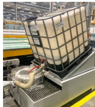
Tilting device to prevent adhesive residues in IBC containers
