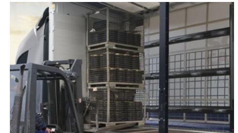
Volumes up to 100 m 3 for automotive logistics: Ability to load pallet cages with positive locking up to 3 m in height.
