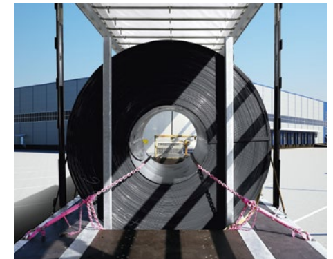
The correct way to transport heavy coils: Combined load security for heavy strip steel rolls.
