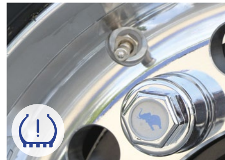
Tyre pressure monitoring system: decreases tyre wear, lowers fuel costs and reduces the risk of breakdowns. The sensor is fitted in the tyre directly on the rim.
