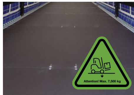
Glued floor: greater stacker axle load of 7.5 tonnes, sealed load area to protect against moisture.
