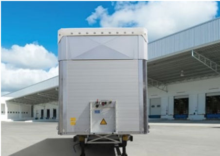
Steel corner stanchions on the bulkhead and rear door increase structural rigidity.
