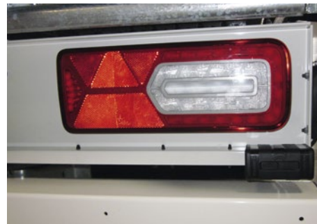
LED rear lights with striking flashing function, energy-saving and less likely to fail. (optional)
