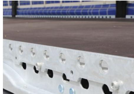
Lashing holes along the entire length of the outer frame for flexible load securing. With optional pallet stop rails.
