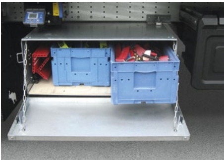
Steel box on the chassis for stowing the load securing equipment.
