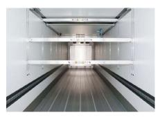
The **multifunctional floor** is easy to clean thanks to the welded base tray. The floor is PIEK-certified, has a longer service life, is non-slip and at the same time lighter.
