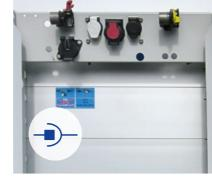
**Coupling sensor:** The tractor unit can be reliably identified by monitoring the supply pressure to the brakes. Trailer-Connect® in the trailer is based on the CTU3 telematics unit which acts as the central control unit.
