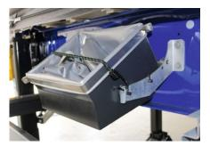
**Grain outlet hopper f**or grain pusher with practical parking position on the chassis or protected in the storage box.
