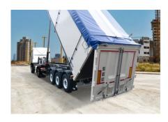
The **curved roller curtain** is easy to handle and can be closed from the ground using the long centre tensioning strap. Emptying with the curtain closed using the swing function of the combi door saves time. The arched shape with stabilising central tube also prevents water from collecting
