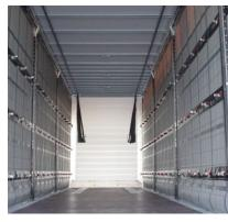
**Body fits to your needs:** 7.1 tonne forklift axle-load tested to DIN EN 283 fully-sealed floor provided as standard. Options for glued floor to reduce damage from water ingress and screws coming loose. Additional options for 7.5 tonne or 9.5 tonne floors.
