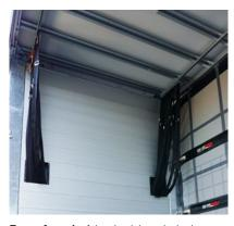
Ease of repair of the aluminium planked bulkhead with steel corner supports for easy side loading and interior bulkhead ram protection. Optional storage compartment for lashing straps on the left and right in the bulkhead.
