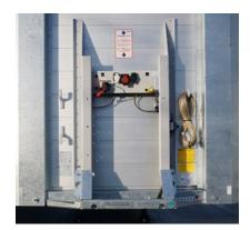
**The C-couplings PLUS** 2 x 7 +1 x 15-pin sockets fitted at the front of the bulkhead fit all tractor units and have an operator-friendly design, reducing the risk of confusing the connections.
