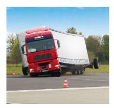
**Fully certified** body according to DIN EN 12642 code XL including beverages transport. Additional high security of goods due to intergrated anti-theft protection 1.8m high in the curtain.
