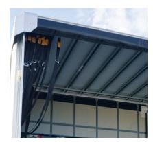
**Fixed Schmitz Cargobull aluminium roof** load restraint options. Our optional restraint straps with recessed tracks on both sides or in the middle prevent loads from slipping, improving safety.
