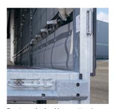
**Easy to repairs door hinges** and hot-dip galvanised corner supports for durability.
