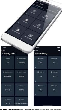
Your personal assistant in the cockpit: beSmart informs the driver about the aggregate load, tyre pressure, brake condition and, with temperature-controlled freight, the settings in the cooling unit, temperature in the cargo area, fuel level, and controls the door locking system. You receive messages on time before critical statuses are reached.
