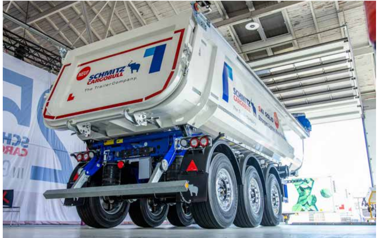
Weighed and given the A-OK: The new troughs and frames for the S.KI and M.KI offer up to 280kg higher payload and can be fitted with a digital on-board weighing system.
