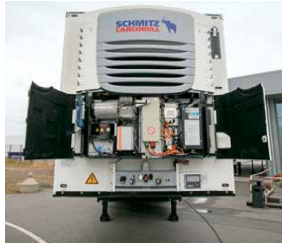
Environmental friendliness: The S.CU ep85 cooling unit was designed for distribution transport and is available in both mono- and multi-temperature variants.
