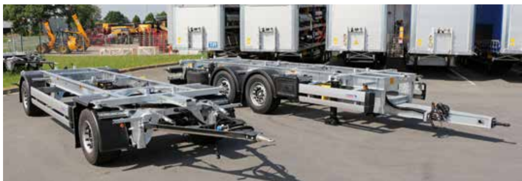
The A.WF and Z.WF swap chassis are suitable for 20' containers.
