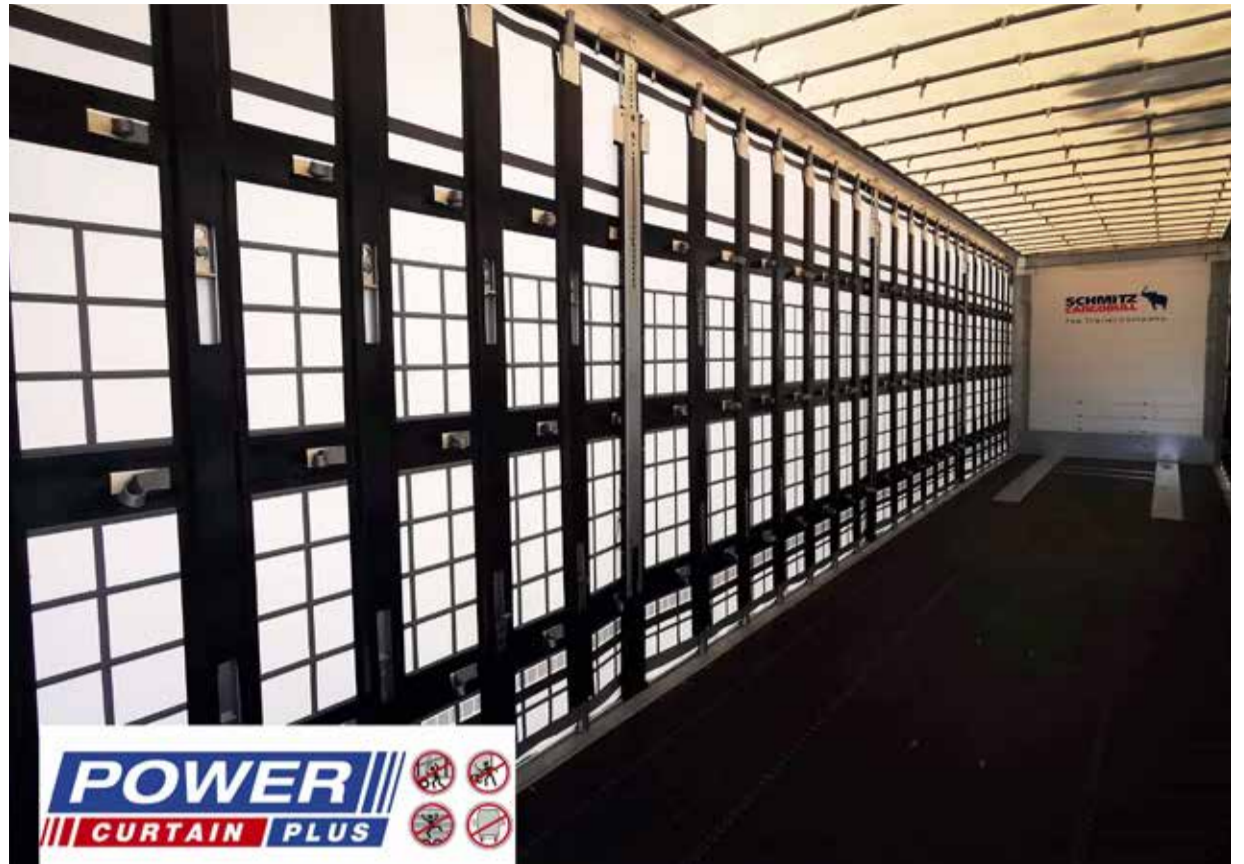
Combined with belts or a load securing tarpaulin, the three rows of load securing loops of the S.CS MEGA DB POWER CURTAIN PLUS develop blocking forces of up to 7,500daN.
