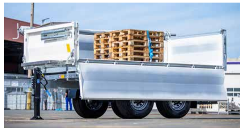
Thanks to lashing points in the trough floor, the Z.KI is also suitable for transporting palletised goods.
