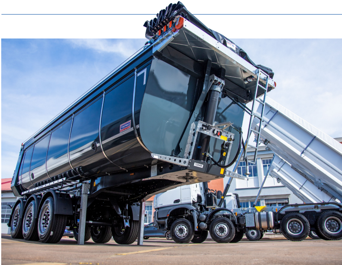
Classic tipper trailer for asphalt transport with electric sliding tarpaulin.
