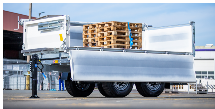
Thanks to lashing points in the trough floor, the Z.KI is also suitable for transporting palletised goods.
