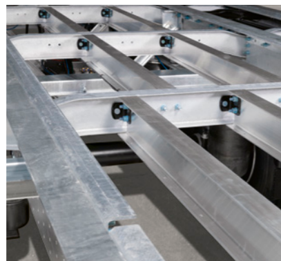
Rolled MODULOS chassis: Corrosion-resistant and easy-to-repair thanks to the bolted and hot-dip galvanised technology.
