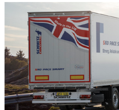
Double leaf doors corrosion-resistant, durable and lightweight. Opened with an opening angle of 270°. Close-fitting to the side wall for good maneuverability.
