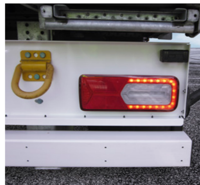
Combined transport: Ferry Lashings* for short-sea transport. For more safety - underride protection according to ECE regulation 58.03.
