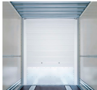
Aluminium bulkhead and Steel kickstrip: protection for cargo and trailer.
