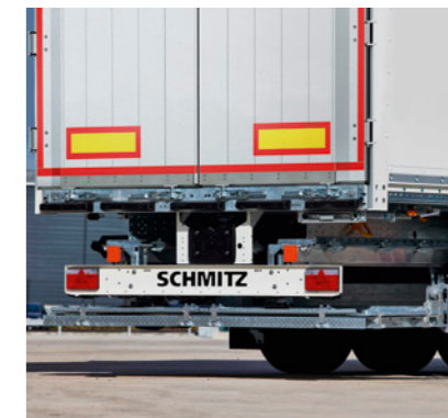
Under-ride tail lift* for loading and unloading without ramp.
