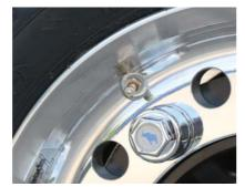
Tyre pressure monitoring system decreases tyre wear, lowers fuel costs and reduces the risk of breakdowns.
