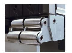
Compression roller bumpers (DRP) are included in the EXECUTIVE PLUS equipment package and protect the rear when approaching ramps.
