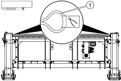
Figure 4: S.KOe COOL rescue disconnection point
