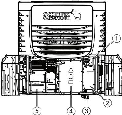
Figure 6: S.CU ep85 cooling unit - Layout of electrical and electronic components (with open doors)
