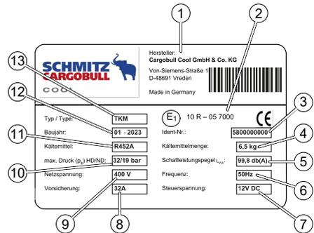
Figure 3: Cooling unit type plate
