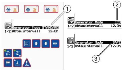
Figure 23: S.KOe COOL – selecting the generator mode
