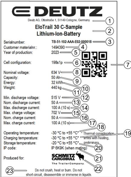
Figure 2: High-voltage battery type plate
