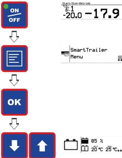
Figure 24: Checking the state of charge
