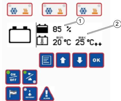
Figure 14: Charge status and temperature
