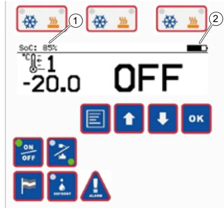
Figure 21: S.KOe COOL – state of charge of the high-voltage battery
