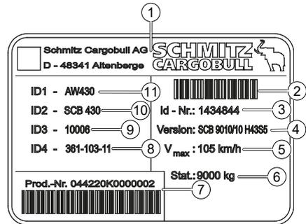
Figure 1: Generator axle type plate
