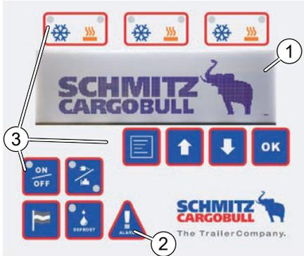
Figure 12: Control panel with start screen (3-chamber version)
