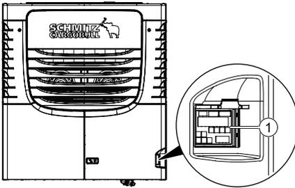
Figure 11: Control panel on the cooling unit
