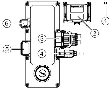
Figure 7: High-voltage battery - overview of plugs and connections
