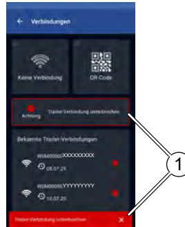
Fig. 56: "Connection failure" display
