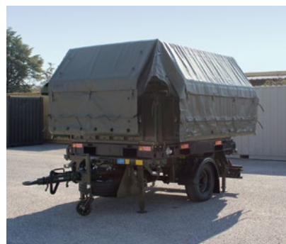
Z.WF 5 MIL with swap chassis platform in the super structure
