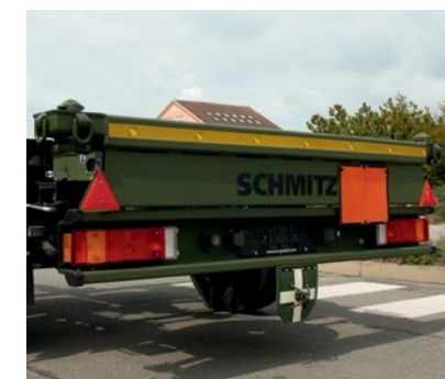
7-chamber lights with integrated camouflage tail light, camouflage brake light left, guide cross with light
