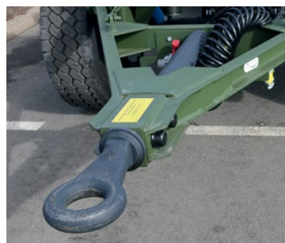
Drawbar according to DIN 74040 with exchangeable NATO drawbar eye according to VG 74059 (drawbar tube extendable by 6 x 100mm)
