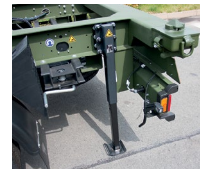
Rear support structure on both sides to stabilise the chassis
