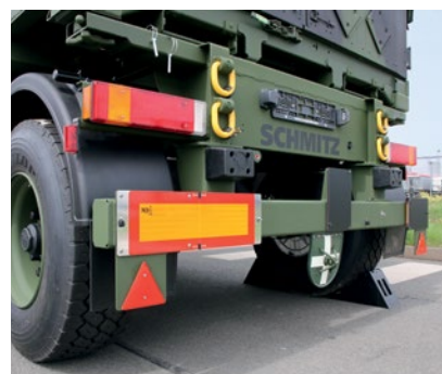
LED side marker lights coupled with turn signal, camouflage tail light and camouflage brake light, guide cross with light, lashing and fastening equipment for rail, ship and airtransport
