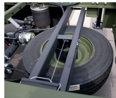
Spare wheel holder in winch design (for one spare wheel)
