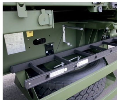
Aluminum ladder 1.80 m incl. holder, spare wheel holder in tub design (for one spare wheel)
