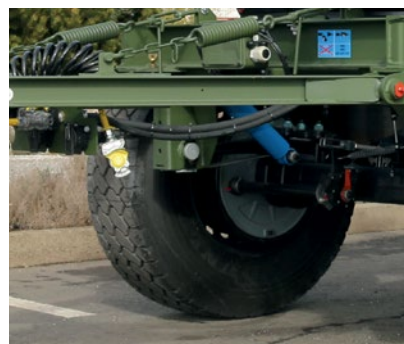
BPW axles with drum brakes
