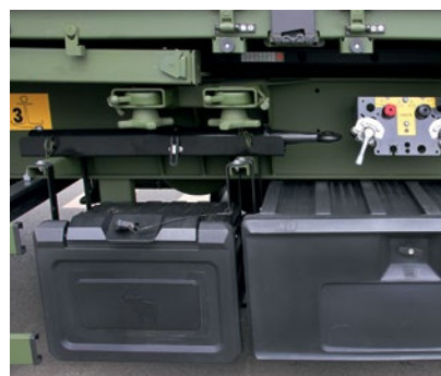
Spare drawbar tube with towing eye according to DIN 74054 (D = 40 mm) in parking position. Toolbox with drawer and shelf and large toolbox to hold camouflage net (Vol: 225 l).
