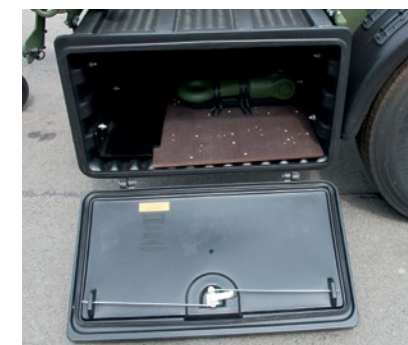
2 toolboxes , optionally 1 toolbox to hold camouflage net (packing size 800 x 600 x 150mm)
