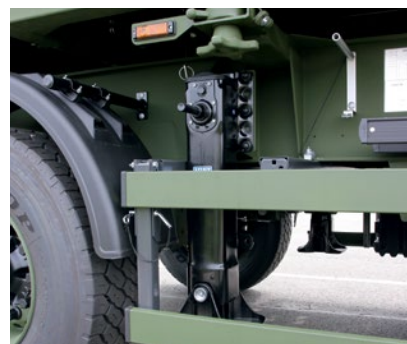
Four steady legs on the chassis for stable off-road positioning
