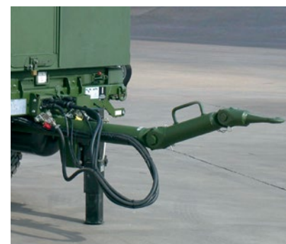
Height-adjustable drawbar with replaceable NATO towing eye (towing eye according to VG74059, DIN D = 40 mm)
