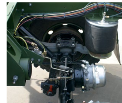
AL-KO axles with drum brakes
