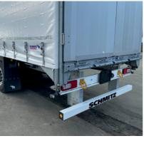
For more safety - underride protection according to ECE regulation 58.03. The forces to be absorbed have almost doubled to 18t.
