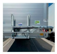
of the light and brake connections thanks to a connection bar that can be pulled out to the side, simplifying and speeding up handling.
