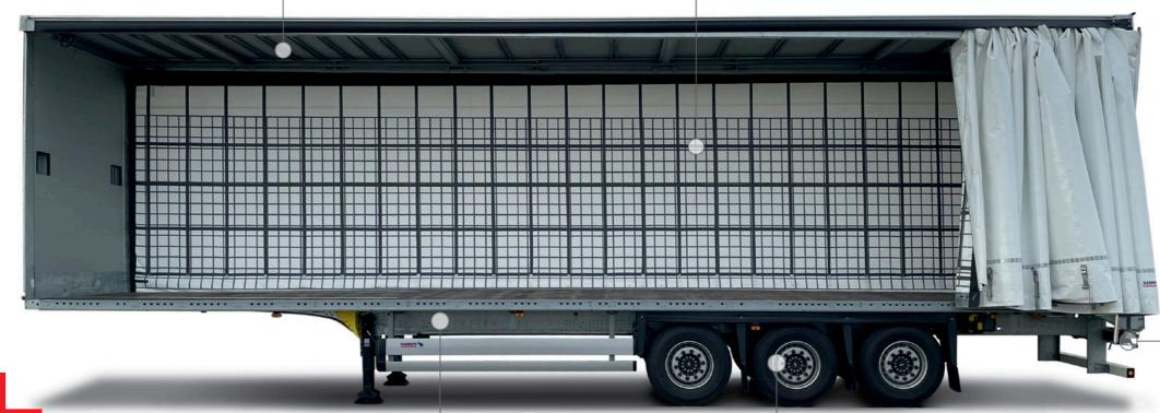
Rolled, galvanised MODULOS chassis
