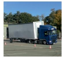
Fully certified structure according to DIN EN 12642 Code XL. High security of the goods through integrated theft protection in the curtain.
