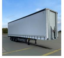
The right body height for every transport application: available in heights of 4,200 mm, 4,400 mm, 4,600 mm and 4,800 mm.
