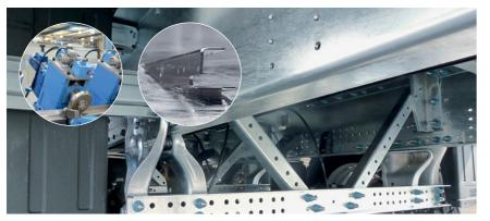
Rolled, galvanised MODULOS chassis - robust, durable and retains its value with low total cost of ownership. Particularly easy to maintain due to bolted and screwed connections. and with a 10-year warranty against rust-through. Hot-dip galvanising offers excellent corrosion protection as well as unmixedrecycling.
