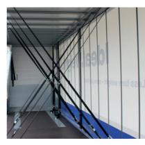
Load securing straps with lashing eyes on the outside or inside centre on both sides prevent the load from slipping.
