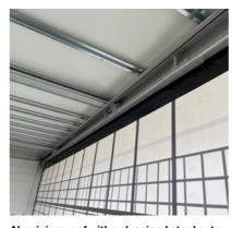
Aluminium roof with galvanised steel outer rail and various load securing options for a lateral loading height of up to 3,200 mm.
