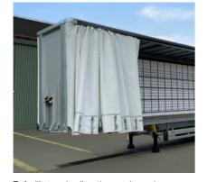
To facilitate unloading, the curtain can be tensioned from both the front and the rear.
