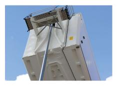
Partially lowered chassis neck area in the floor assembly of the body for a lower body loading height and a lower overall height.
