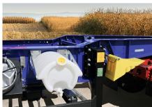
The offset in the neck area of the chassis (stepframe) enables a reduced loading height.
