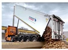
Increased manoeuvrability due to low wheelbase. Ideal tipper semi-trailer for the efficient transport of agricultural products in confined spaces such as narrow field tracks. Thanks to its voluminous equipment, it offers the largest possible loading space with maximum payload, ideal for goods with low bulk density.
