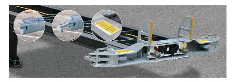
**PIN locking** against twisting on two pairs of container beams as standard locking.
