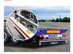
New design: **Extendable underride guard** for 45' containers is easier and safer to handle with no easy to lose, loose parts.
