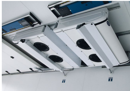
Additional ceiling evaporator* for MultiTemp versions and trailers in through-loading trains.
