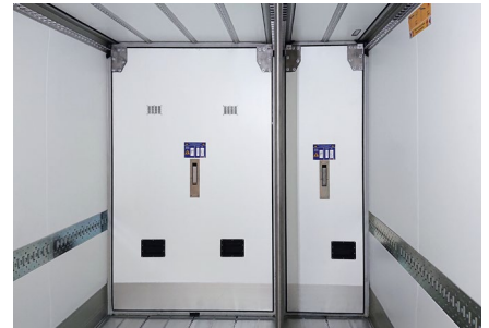
Sliding partition wall* made of vapour diffusion-tight FERROPLAST® : Fast, variable MultiTemp partitioning; optionally available for 1/3 and 2/3 partitioning or as a continuous wall.
