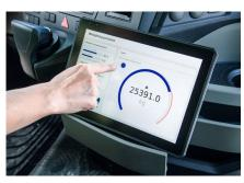
The factory-calibrated **on-board weighing system\*** is ready for use in 5 seconds and can be operated via the screen or beSmart app. A stationary checkweigher does not need to be approached, the weighing data is available immediately.
