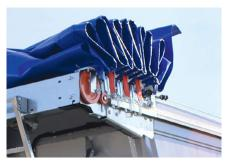
The **sliding roof\*** enables time-saving opening and closing. Available in a manual or electric version, operated by remote control.
