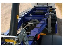
The torsion-resistant steel chassis with improved corrosion protection in a painted or galvanised finish ensures the best possible value retention.
