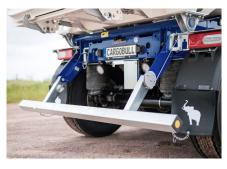
The folding underride guard offers high ground clearance for use on road pavers. It can be operated manually and is optionally available with a spring mechanism for easy handling or as a pneumatic version for increased safety and time savings.
