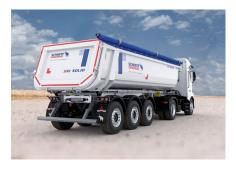
The roller curtain serves as a simple and costeffective body cover against moisture and drifts and reduces air resistance. The optional sliding roof enables time-saving opening and closing by remote control.
