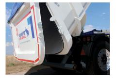
The surface-mounted swing flap is suitable for partial unloading and is optionally available with a slide. Swing flaps with chute, combination doors or hydraulic rear wall flaps extend the range.
