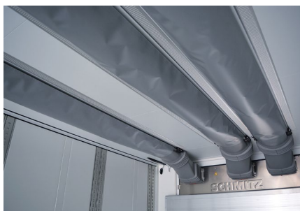
Efficient air flow: With three air ducts and a collision-resistant hood, the tempered air is evenly distributed throughout the body, ensuring low energy consumption.
