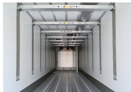
Reliable load securing: The S.KOe COOL offers numerous equipment options customised to your transport needs. An intelligent system of load securing rails make loading and unloading safe and easy.
