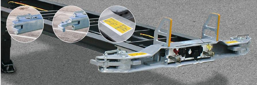
**PIN locking** against twisting on two pairs of container beams as standard locking.
