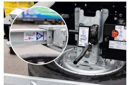
**New labelling** on locks and extensions for reliable identification of the different loading positions, supported by a loading plan and operating videos via QR code.
