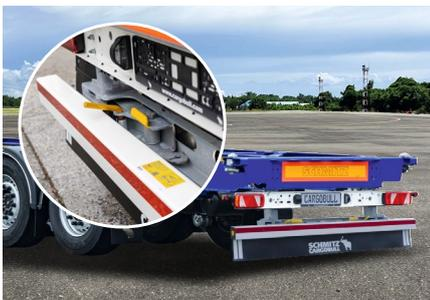
New design: **Extendable underride guard** for 45' containers is easier and safer to handle with no easy to lose, loose parts.
