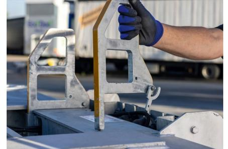
Easily replaceable **container guides** for containers on the front beam.
