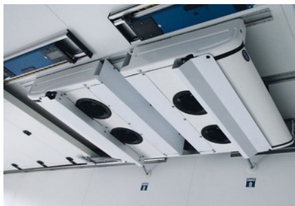
Additional roof evaporator* for MultiTemp versions and trailers in through-loading trains.
