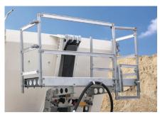
The **working platform** is used to operate the roller curtain and is equipped with a non-slip floor, body entry aid and parking position for the hydraulic hose
