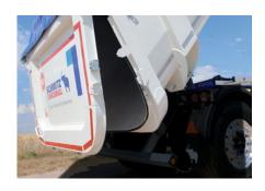
The surface-mounted **swing flap** is suitable for partial unloading and is optionally available with a slide. Swing flaps with chute, combination doors or hydraulic rear wall flaps extend the range.
