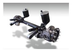
The **Schmitz Cargobull axle units** consist of optimally harmonised, high-quality components. MRH air suspension (multi-ride-height): Ideal for lowering the centre of gravity when unloading – Even more robust, yet lighter
