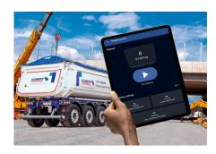
The factory-calibrated **on-board weighing system\*** is ready for use in 5 seconds and can be operated via the screen or beSmart app. A stationary checkweigher does not need to be approached, the weighing data is available immediately.
