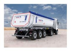
he **roller curtain** serves as a simple and costeffective body cover against moisture and drifts and reduces air resistance. The optional sliding roof enables time-saving opening and closing by remote control.
