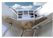
Interior lighting for aluminium volume skips enables cleaning or handling with palletised freight even when the top is closed and ensures better illumination during night-time operation.
