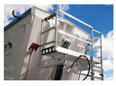
Safe and practical: the **height-adjustable working platform** with non-slip floor, access aid for the skip and parking position for the hydraulic hose
