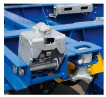
With 2x20' loads the two **KLAPP** LOCKs serve to lock the rear end of the front container.
