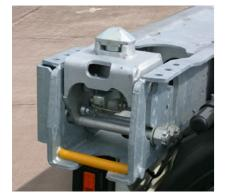
Two STEP LOCKs®\* on the rear extension allow you to adjust your semitrailer container chassis in a matter of moments.
