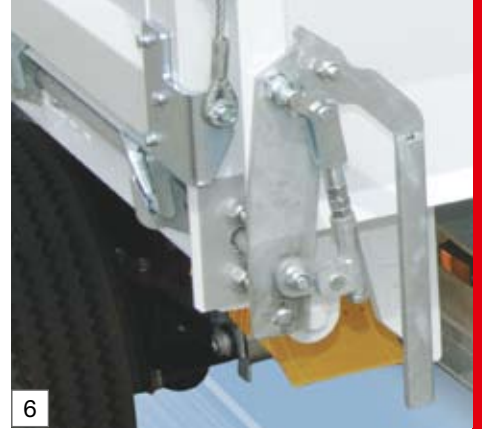
Central lock for swinging side panels on the bulkhead with over-centre helper spring
