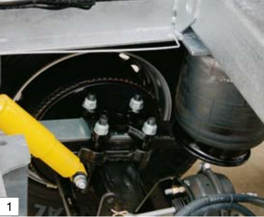
Schmitz Cargobull air suspension with drum-braked axle (wheel offset 0 mm)
