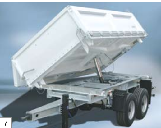
Steel tipper body with one-piece continuous floor plate from buckling and wear-resistant steel HB 450
