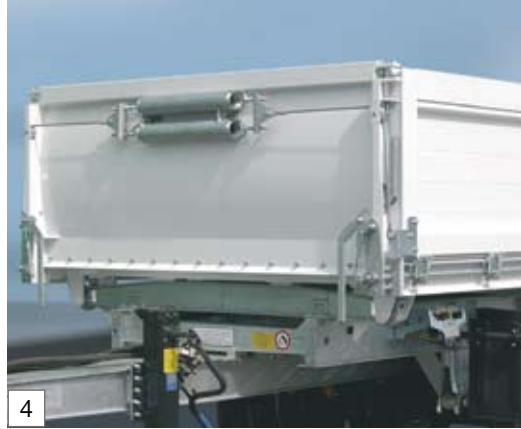
Dropside lifting aid on both sides by spring relief (only on aluminium dropsides)
