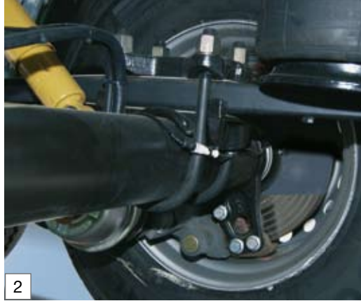
MRH pneumatic suspension with disk-braked axle, large disk dia. 430 mm (wheel offset 120 mm)
