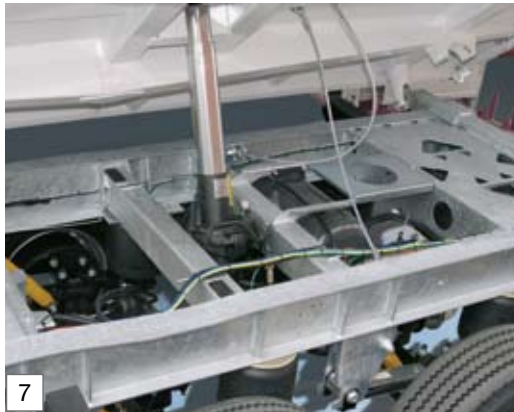
7 Frame made from high quality welded steel construction, hot galvanised, 3-sided tipping system with underlying cylinder and operating pressure 225 bar
