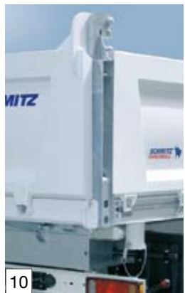
Corner stanchions from fine-grain galvanised steel, bolted, adjustable using eccentric cam
