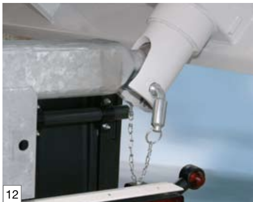
Tipping bearing with cross-over protected steel lock
