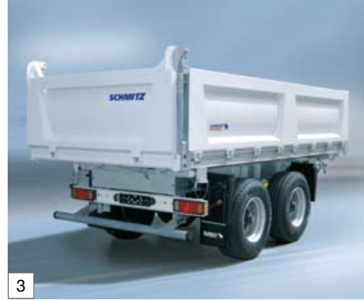
Side undivided steel tank diaphragm dropside, from buckle- and wear-resistant steel, supported in a swinging manner
