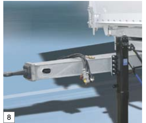
8 Straight welded tow bar, length and height adjustable, spindle support leg, maintenance-free
