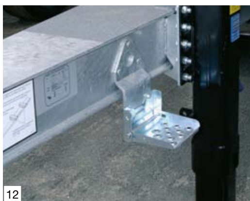
Platform including roller tarpaulin, boarding point on the tow bar with anti-slip surface on the tow bar
