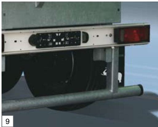
9 Underride guard, can be folded down for road repair use
