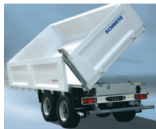
Steel tipper body with single-part floor plate
