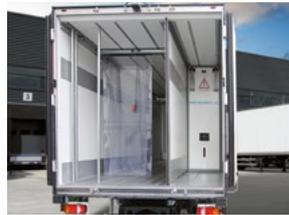
A variety of versatile fittings for multi-compartment vehicles and different temperature zones.
