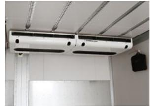
Optimised evaporator in the interior ideal for multi-temperature vehicles.
