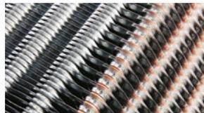
The number of cooling ribs at the front of the evaporator has been reduced to prevent them from icing up.
