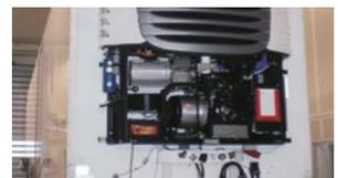
The transport refrigeration unit successfully covered 500,000 km of endurance and load tests at the Schmitz Cargobull Validation Centre.
