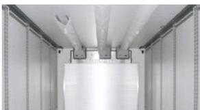
The intake duct for the evaporator is protected behind the circulation wall.
