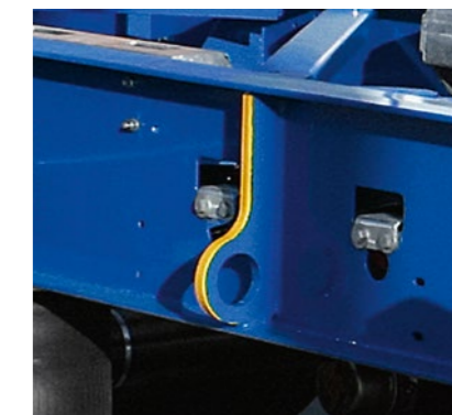
The container trailer chassis can be equipped with ferry lashings * for use with ferry transport.
