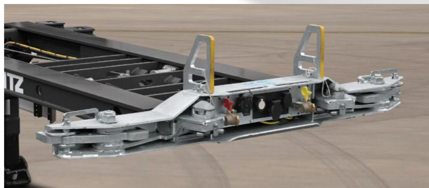
For carrying 45' EU containers: the patented MULTI LOCK ® locking mechanism on the mechanical front extension for total versatility.
