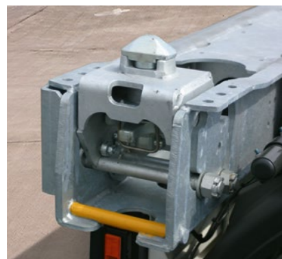
Two STEP LOCKS ® on the rear extension allow you to adjust your semi-trailer container chassis in a matter of moments.
