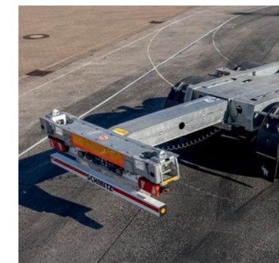
New: Damped rear extension moves pneumatically to the selected locking position and brakes gently.
