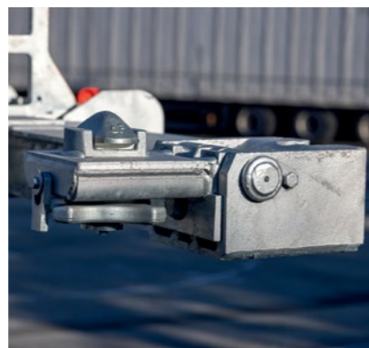
Folding lock on the rigid front beam in the twist lock position .
