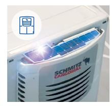
Solar panel\* protects the starter battery from deep discharge and thus from damage. Battery life is increased and comfort functions are available for longer
