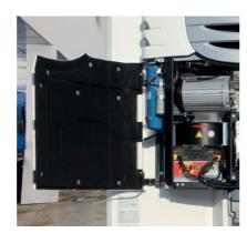
Silent-Kit is installed as standard in the casing of every cooling unit S.CU and reduces drive
