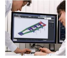
Extra-LIGHT-chassis: FEM-designed for maximum torsional rigidity and safety while maximising the payload.
