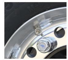
Tyre pressure monitoring system: decreases tyre wear, lowers fuel costs and reduces the risk of breakdown.
