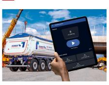
The ex-works calibrated on-board weighing system\* is ready for use in five seconds and can be operated via the screen or beSmart app. There is no need to drive up to a stationary control scale, as the weighing data is available immediately.
