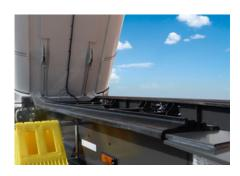
Low centre of gravity and optimal driving dynamics: the rounded steel tipper body fits perfectly on the rubber mountings of the chassis. The wide, flat floor design of the aluminium box and rounded steel tipper bodies ensures a low centre of gravity and makes cleaning the tipper body easier.
