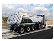
Cladding of the rounded steel tipper body made of floating insulated panels – individual segments can be quickly replaced in the event of external damage.werden.
