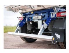
The **foldable underride guard** offers high ground clearance and can be operated manually. It is optionally available with a spring mechanism for easy handling or in a pneumatic version for increased safety and time savings.
