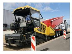
High-quality, temperatureresistant cover The rolling tarpaulin is a simple and cost-effective tipper body cover that protects the load, prevents the mix from cooling due to trapped heat and reduces air resistance. The optional sliding roof enables time-saving opening and closing by remote control.
