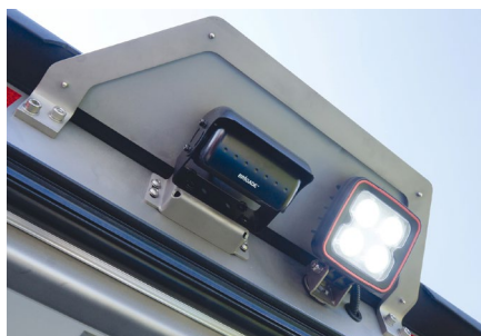
The reversing camera* and LED work lights* ensure additional safety and prevent damage when reversing, docking on ramps and manoeuvring.
