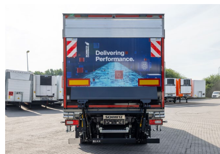
Tail lift as rear end. A double-wing rear door with a tail lift that can be folded forward or lowered is standard.
