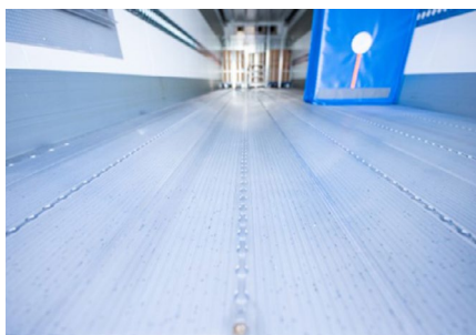
Airline floor* with optimised slip resistance and perforated strip for load securing: welded floor pan fulfils hygiene regulations, is quick to clean and saves time.
