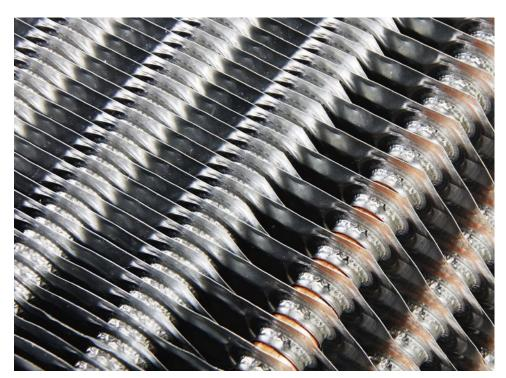
Up to 50% fewer defrosting cycles thanks to improved evaporator design: the number of cooling ribs at the front of the evaporator for the Schmitz Cargobull S.CU transport refrigeration unit has been reduced to prevent them from icing up.
