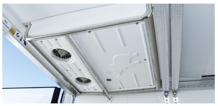
Powerhouse beneath the roof: The powerful technology of the Schmitz Cargobull additional roof evaporator ensures even temperature distribution. The heat exchanger with a large evaporator surface is distinguished by high performance and low defrosting cycles thanks to minimal ice formation.
