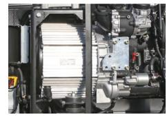
Improved operational reliability due to optimised heat management and the additional hermetic sealing of the generator.
