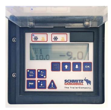
The control panel on the refrigeration unit can be used to configure all the important settings, such as the precise temperature specification and setpoints.
