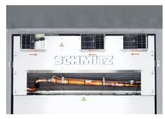
Three fans on the evaporator for optimum air distribution in the body.
