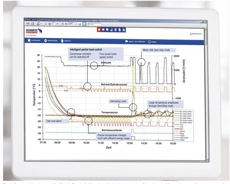
The intelligent partial-load control of the Schmitz Cargobull refrigeration unit minimises temperature fluctuations. Avoiding peaks ensures the even, exact cooling of all the temperature zones independently of each other.
