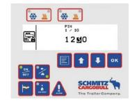
The control panel is secured against unauthorised access by a four-digit PIN that you can individually configure per trailer.
