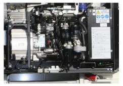
Common rail technology allows fuel injection and ignition time to be individually controlled to optimise performance and consumption.
